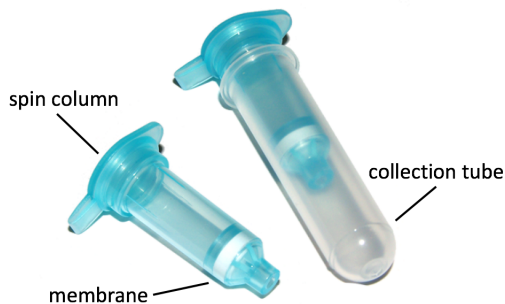
Figure 1: Spin columns. On the left is shown a spin column by itself, and on the right is a spin column in a collection tube. When enough force is applied, a liquid sample will flow through the white membrane and collect in the clear collection tube. These membranes are designed so that certain cellular components are captured or bind to the membrane while others are allowed to flow through. Such selectivity is essential for isolating DNA from samples.
