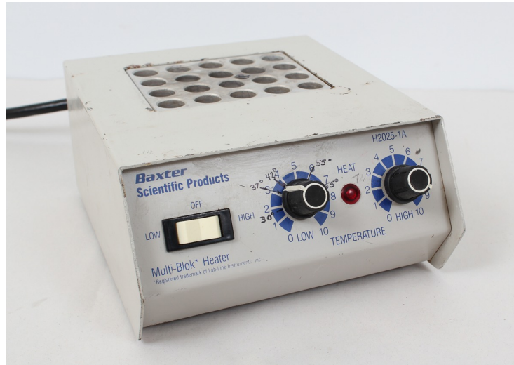
Figure 4: Heat block. An instrument used to keep samples at a particular temperature.
