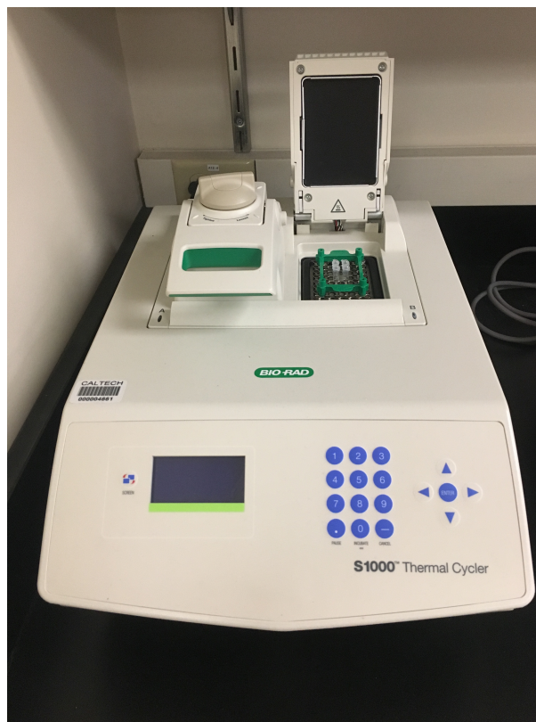
Figure 9: Thermocycler – The thermocycler has two chambers (labeled A and B) into which we can insert your PCR tubes. Using the buttons and display on the front, we can then program the thermocycler to incubate the tubes at specific temperatures for specified lengths of time.
