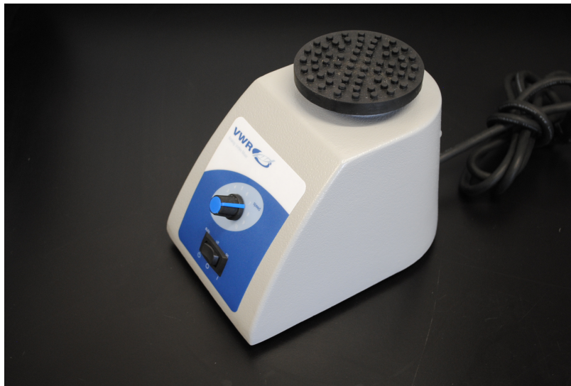
Figure 3: Vortexer. A device used to vigorously shake samples. Simply press your tube on the black rubber platform, and the platform will begin to shake. The speed of the vortexer can be changed by turning the knob, but we will be using it at the maximum speed (indicated as 10 on the vortexer).
